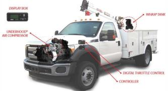
Engineered for trucks and commercial vans, the UNDERHOOD40 delivers up to 40 CFM at 100% duty cycle while freeing up truck deck and cargo space, and decreasing GVW by up to 290 lb.
