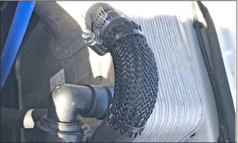
Figure 93 — Installing the secondary coolant hose
