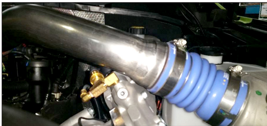
Figure 103 — Installing the CAC hoses
