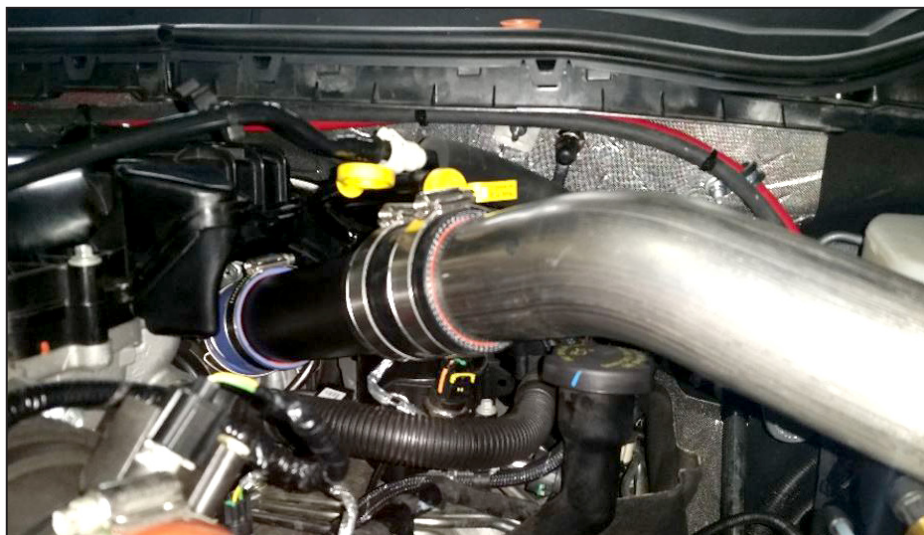
Figure 102 — Installing the CAC hoses
