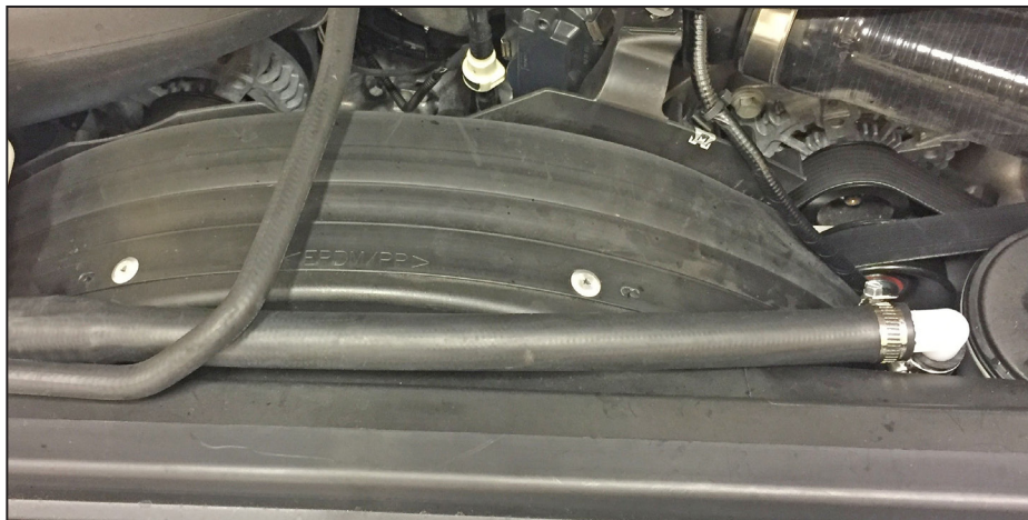
Figure 94 — Installing the secondary coolant hose
