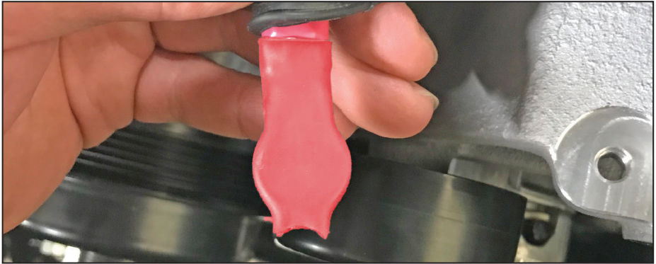
Figure 39 — Isolate secondary alternator harness
