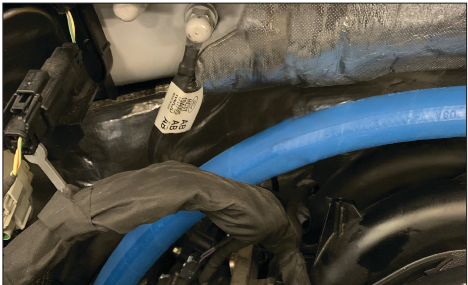
Figure 52 — Install hose routing bracket (blue hose shown for clarity)
