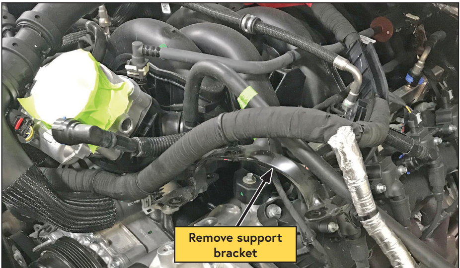
Figure 4 — Remove mounting bracket (dual alternator only)
