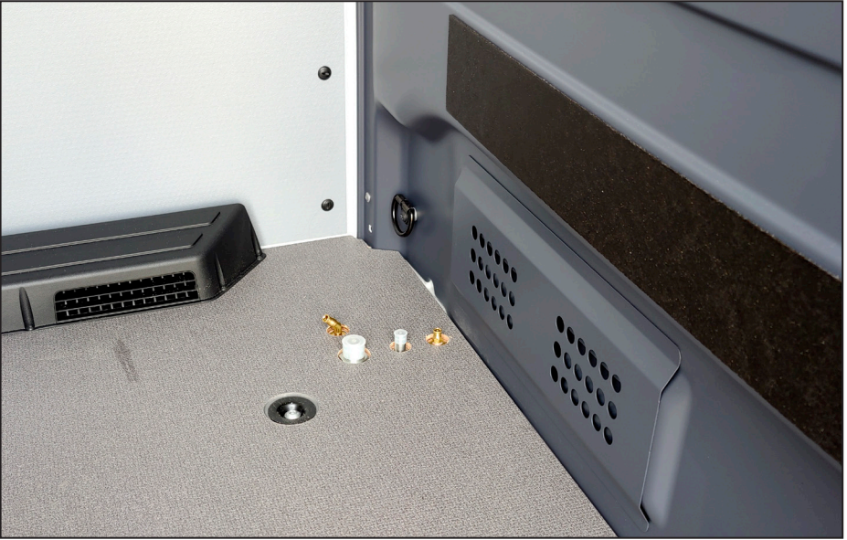
Figure 20 — Bulkhead fittings installed (interior view) (some applications may not include subfloor)
