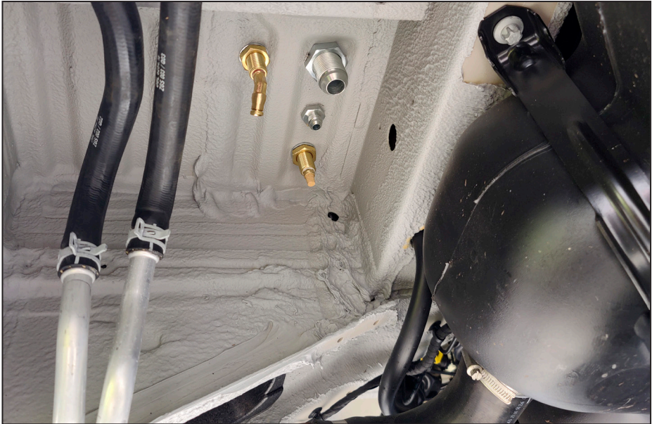
Figure 21 — Bulkhead fittings installed (exterior view)
