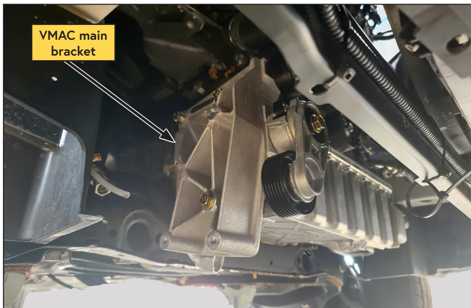
Figure 5 — VMAC main bracket installed (idler installed in later step)
