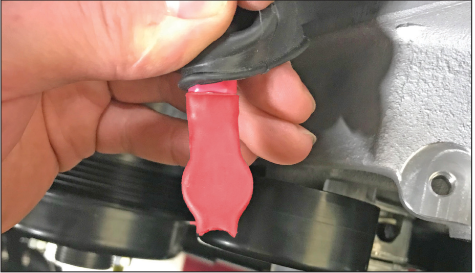
Figure 15 — Isolate secondary alternator harness
