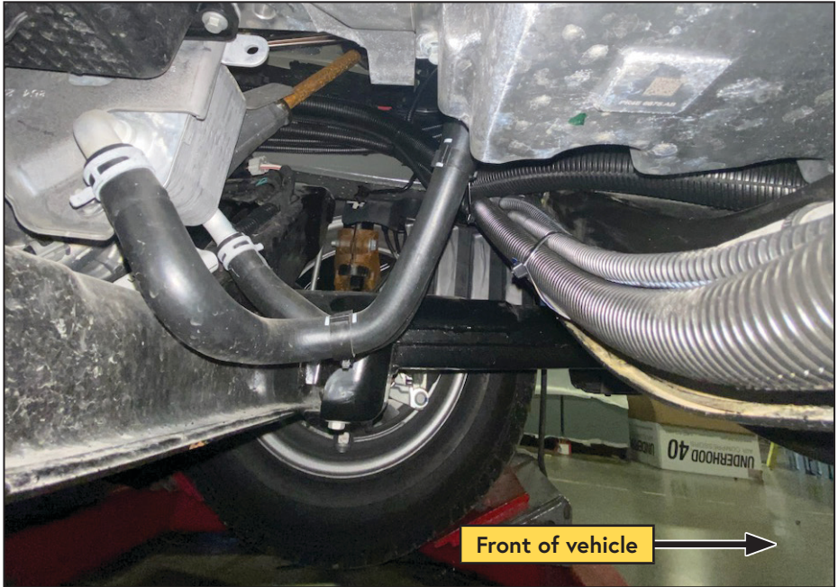
Figure 34 — Route hoses under the oil pan
