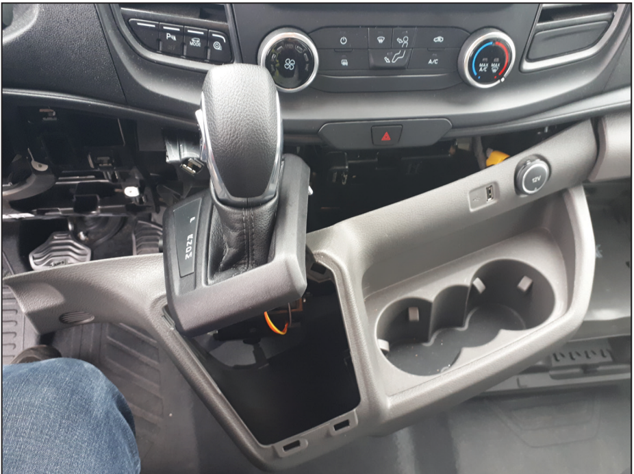
Figure 50 — Rotate shifter console
