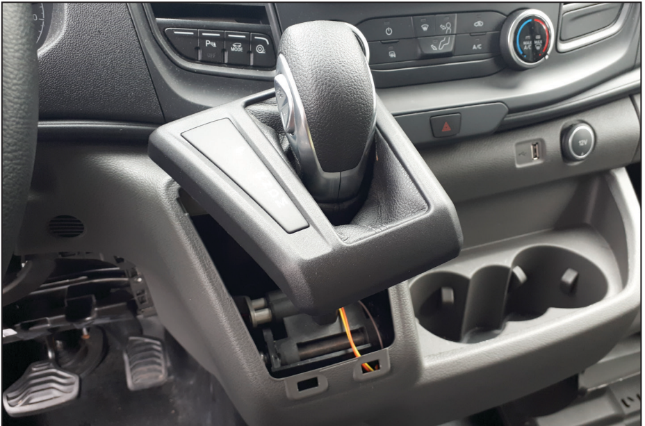
Figure 48 — Remove gear indicator panel
