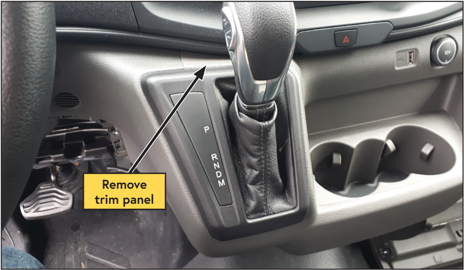
Figure 49 — Remove shifter console
