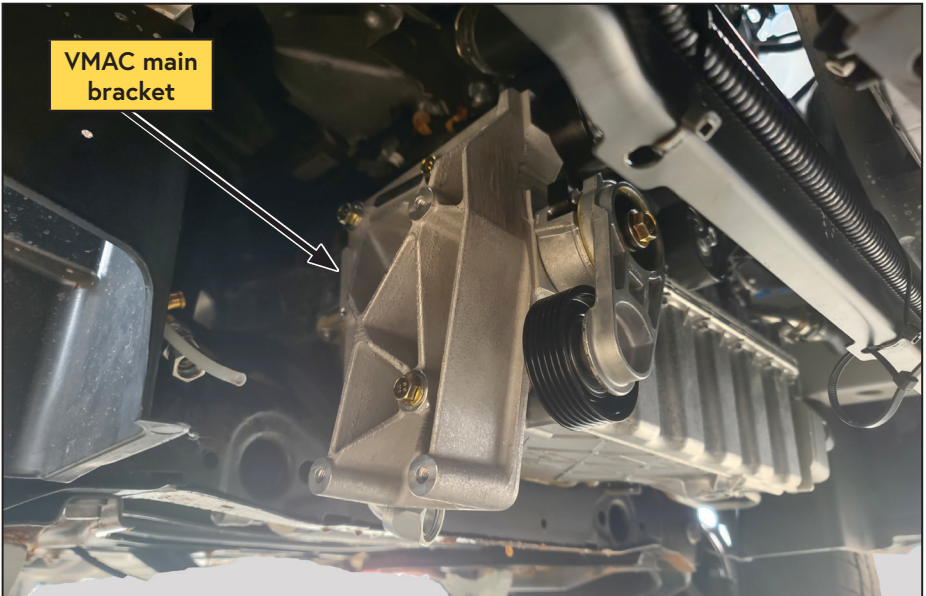
Figure 10 — VMAC main bracket installed (idler installed in later step)
