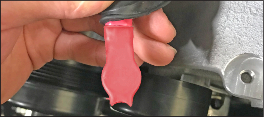
Figure 7 — Isolate secondary alternator harness
