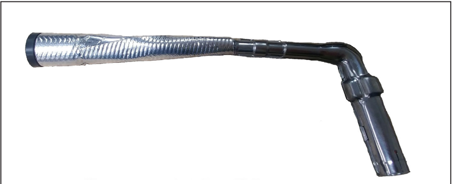
Figure 10 — Apply heat wrap
