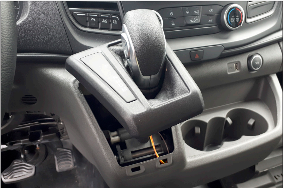
Figure 48 — Remove gear indicator panel
