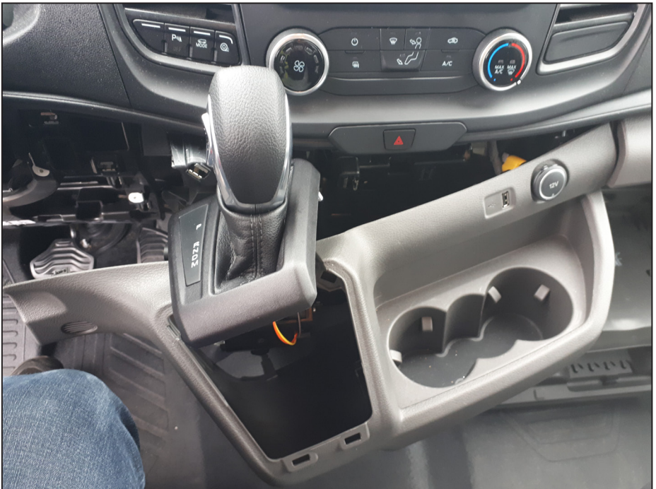
Figure 50 — Rotate shifter console
