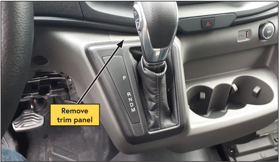
Figure 49 — Remove shifter console
