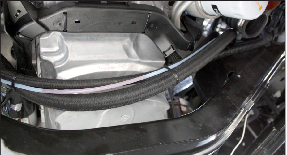
Figure 34 — Route hoses under the oil pan
