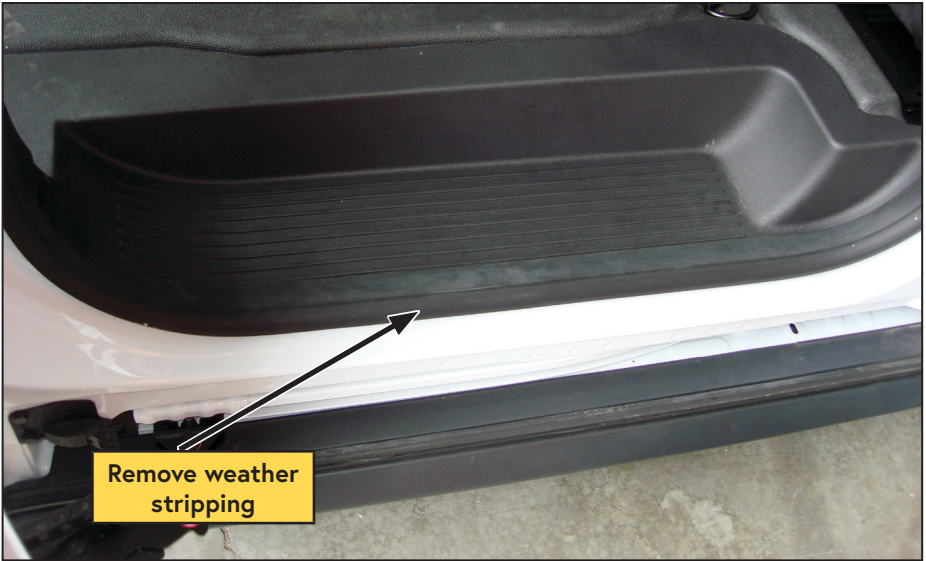
Figure 18 — Remove plastic step
