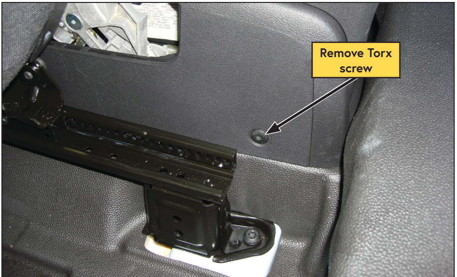
Figure 49 — Remove centre console
