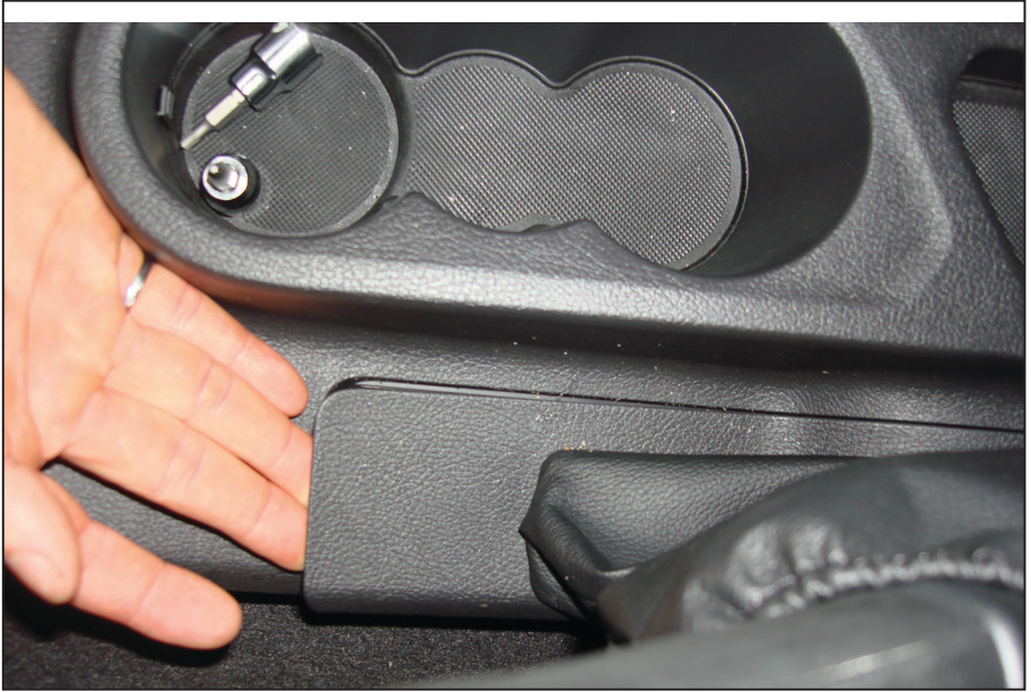
Figure 48 — Remove centre console
