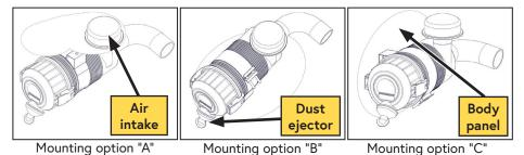
Figure 69 — Installing the remote air intake housing
