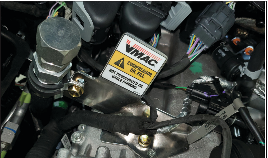
Figure 28 — Install oil fill hose
