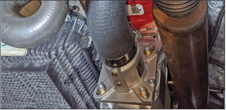
Figure 37 — Installing the remote air intake housing
