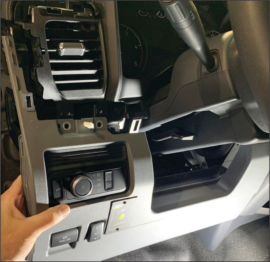
Figure 46 — Remove lower dashboard
