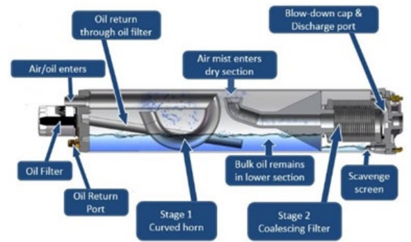
Figure 6: Primary separator tank
