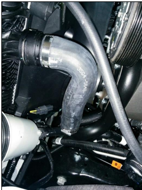
Figure 24 – Installing the upper radiator hose
