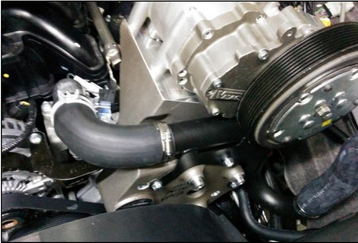
Figure 25 – Installing the upper radiator hose
