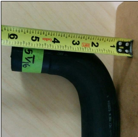
Figure 14 – Modifying the top radiator hose
