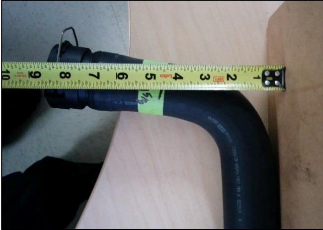
Figure 13 – Modifying the top radiator hose
