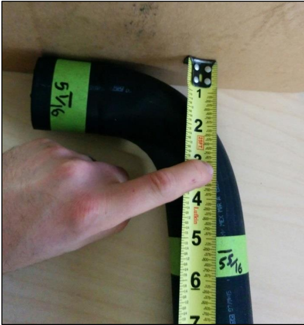
Figure 15 – Modifying the top radiator hose
