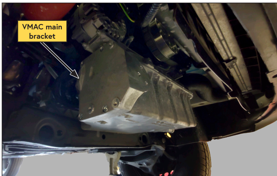
Figure 10 — VMAC main bracket installed
