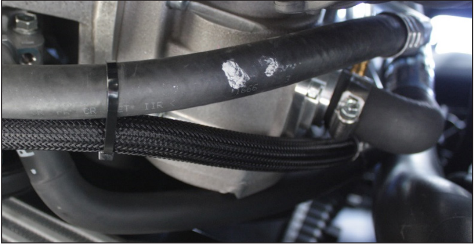
Figure 25 — Adjust A/C hoses
