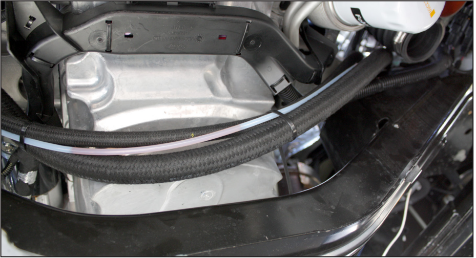
Figure 44 — Route hoses under the oil pan
