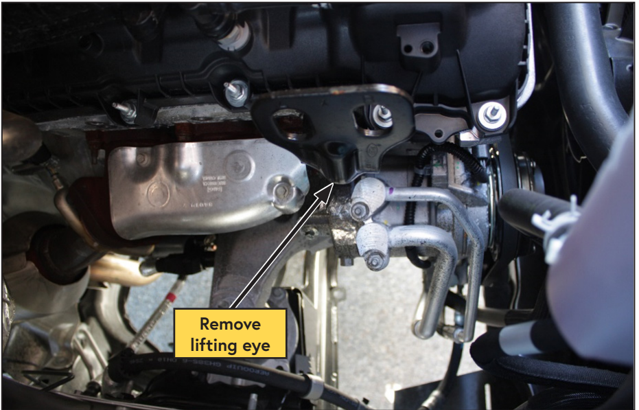
Figure 11 — Remove engine lifting eye and turbo outlet
