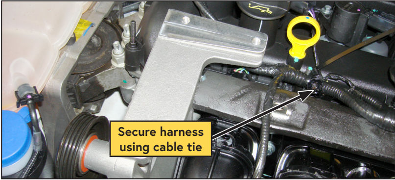
Figure 22 — Secure harness
