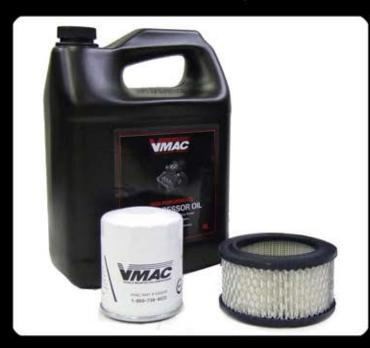
VMAC recommends servicing your Air Vantage 500 Air Compressor System every 500 hours or 1 year, whichever comes first regardless of whether the compressor is being used. VMAC also recommends replacing the Coalescing Filter every 1,000 hours. Service Kits and replacement parts are available.
